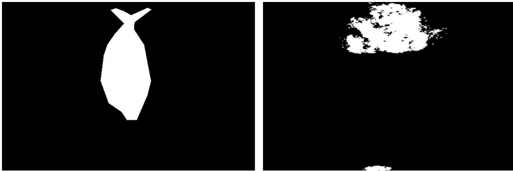
Figure 5.10: Comparison of a mask from a human-drawn polygon to that of an inference of a bucket of fish
