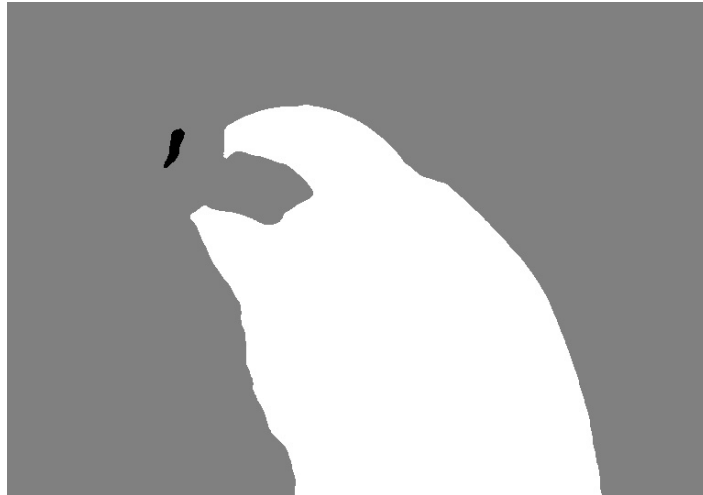
Figure 4.11: Mask of an example image after the nozzle has been removed by superimposing a background mask.
